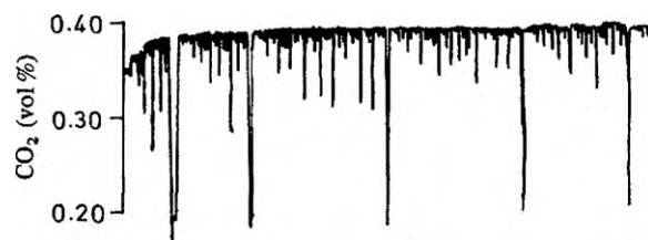
Fig. 1. Aperiodic oscillations observed during carbon monoxide oxidation over a 20 mg sample of a NaX zeolite catalyst containing 4.4% palladium ( \emptyset of zeolite crystallites is 50 \mu\text{m} , \emptyset of Pd clusters is 10 nm). Initial catalyst temperature T_0 = 453 K. Feed CO concentration is 0.4 vol.%. [10].
